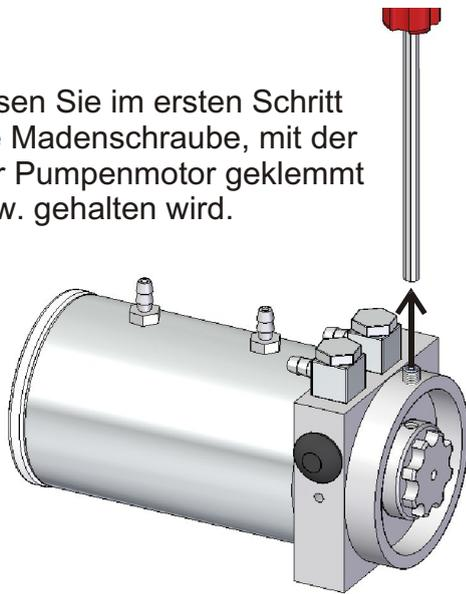
Lösen the worm-screw which is used to hold/clamp the pump-motor and remove the old brushed pump-motor.
