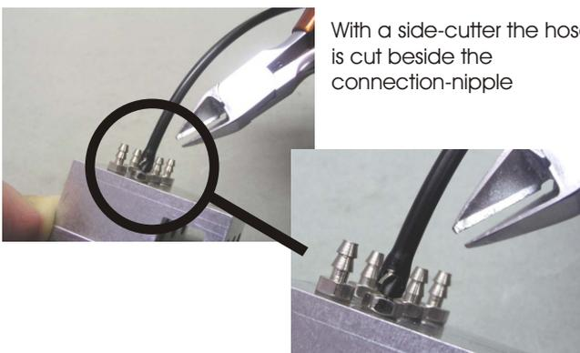
With a side-cutter the hose is cut beside the connection-nipple
