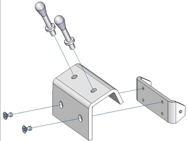
In the second step please prepare the control-panel by screwing in the joysticks and mount a connecting-plate to it using countersunk screws DIN-965 M1.6 length 3mm
