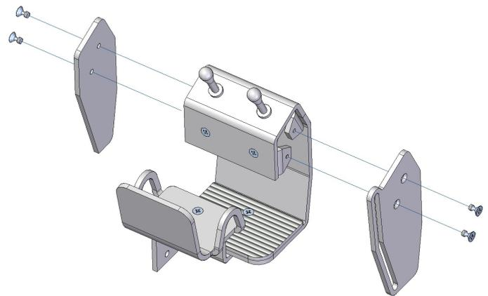
Finally mount the side panels again using countersunk screws DIN-965 M1.6 length 3mm
