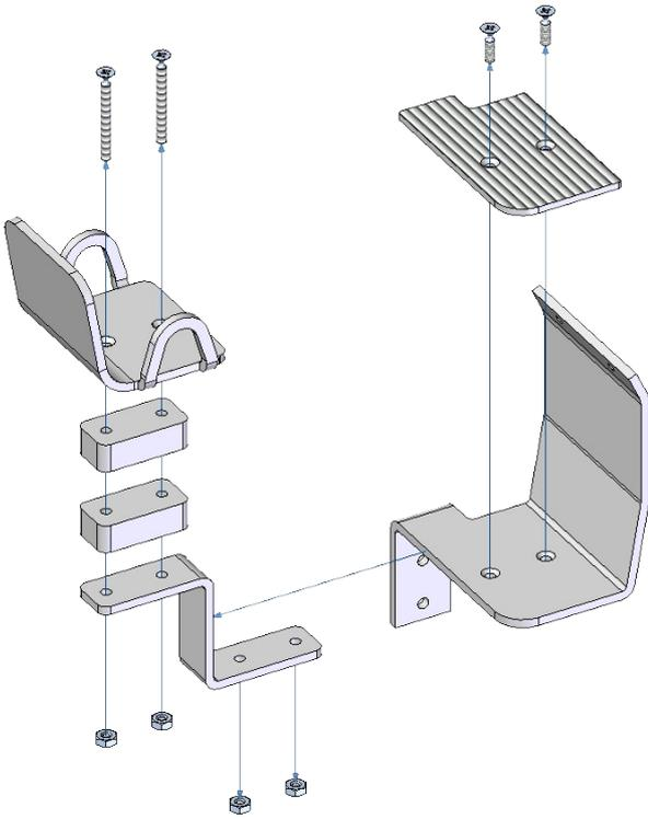
First the seat is mounted to the holder using countersunk screws M2 length 16mm (or M2 length 8mm if only 1 spacer is used) and nuts M2. Depending on the scale of your driver-dummy you can differ with count of the spacer-parts below your seat. Then the unit of holder and seat will be mounted together with the checkered plate to the platform using countersunk screws M1.6 length 6mm and nuts M1.6
