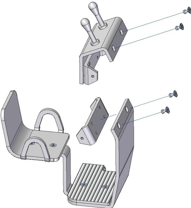
Then again using screws DIN-965 M1.6 length 3mm mount a connecting plate to the unit pre-assembled in the first step and after that mount the unit from the second step also to it.
